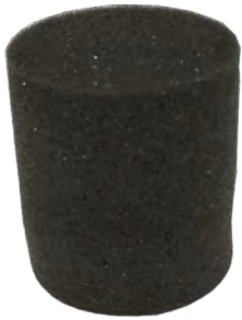
Standard projectile material - Polyurethane.
