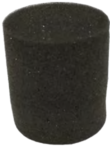
Standard projectile material - Polyurethane.
